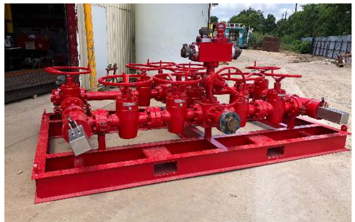
3 1/16 inch 10,000 psi choke manifold built in Houston, TX
